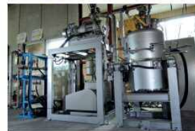
30kg vacuum induction furnace for R&D melting
