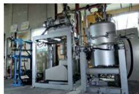
30kg vacuum induction furnace for R&D melting
