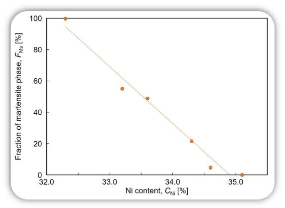
Relationship between area fraction of martensite phases formed during cryogenic treatment and Ni contents in the Fe-Ni based low thermal expansion alloys.
