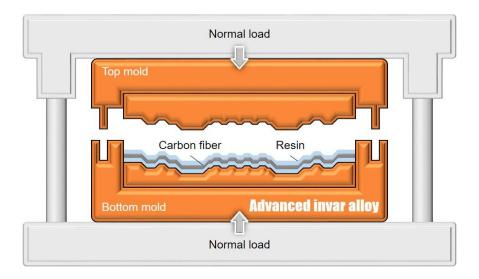
Press forming with the advanced invar alloy molds that allow mass production of the small CFRP components with intricate structure.
