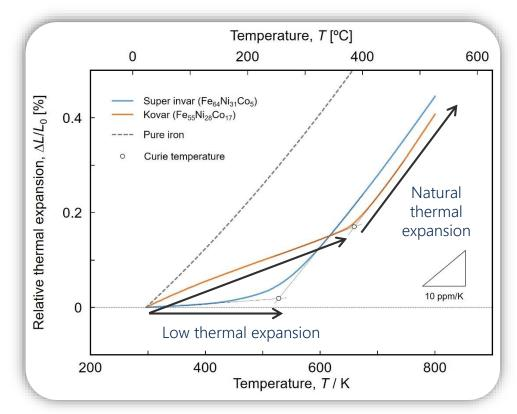
Thermal expansion curves obtained from super invar ( $Fe_{64}Ni_{31}Co_5$ ) and kovar ( $Fe_{55}Ni_{28}Co_{17}$ ) alloys. For comparison, a curve of pure iron is also shown by dotted line.
