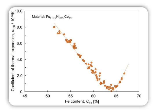
Relationship between average coefficients of thermal expansion and Fe content. The average coefficients of thermal expansion were measured between room temperature and 100°C.
