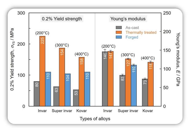
0.2% yield strength and Young's modulus of the as-cast and the thermally treated invar, super invar and kovar alloys. For comparison, those of the forged alloys were also shown.
