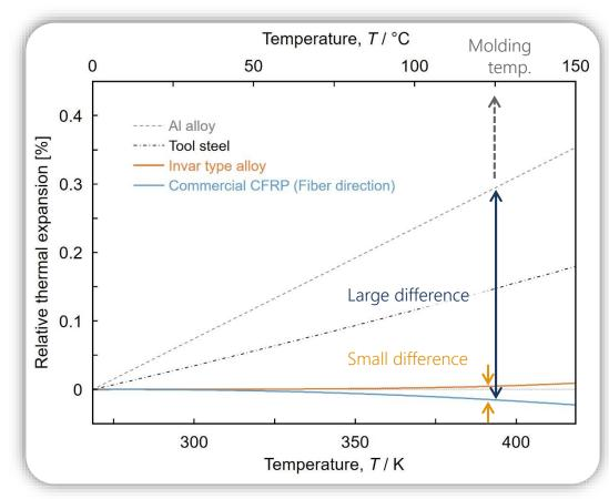
Comparison of relative thermal expansion curves to a dimension at room temperature between tooling materials.
