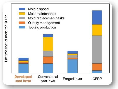
Summary of lifetime cost in each tooling material for small CFRP component with an intricate structure.
