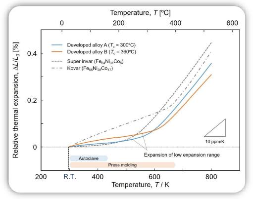
Thermal expansion curves obtained from newly developed alloys by controlling Curie temperature. For comparison, the curves of conventional super invar and kovar alloys are also shown by dotted lines.
