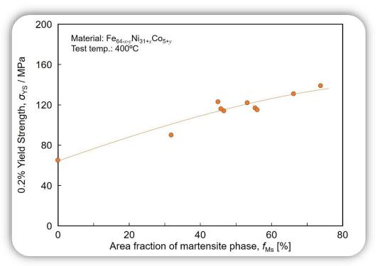
Relationship between 0.2% yield strength after austenite transformation and the area fraction of martensite phases formed during cryogenic treatment by liquid nitrogen in the  $Fe_{64-x-y}Ni_{31+x}Co_{5+y}$  alloys.
