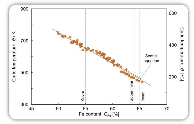
Relationship between Curie temperature and Fe content in the  $Fe_{64-x-y}Ni_{31+x}Co_{5+y}$ . Curie temperatures were estimated from inflection points of thermal expansion curves.
